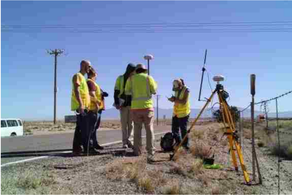
Figure 9. An illustration of the RTK system in a base/rover configuration.
