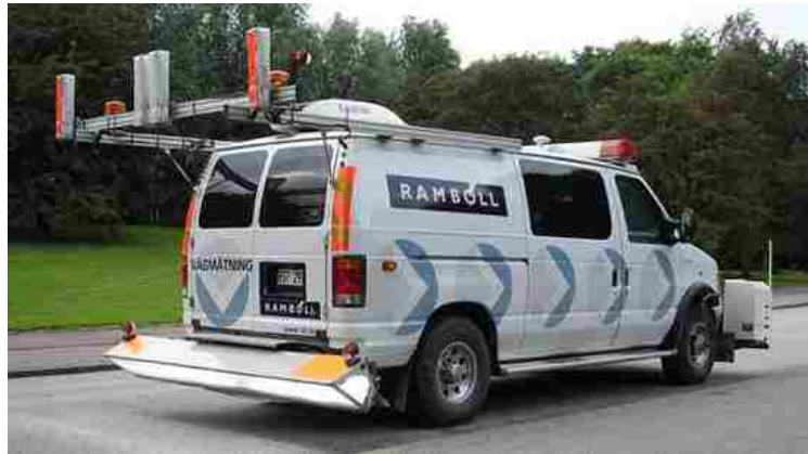
Figure 4. Automatic pavement surface distress evaluation system.
